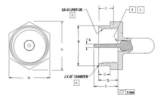
Figure 1 - Male 'F' Terminator Physical Requirements
