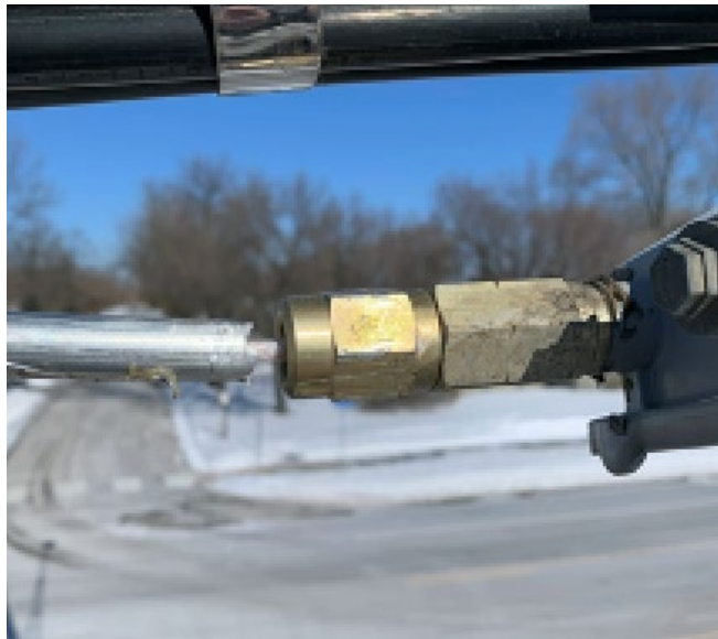
Figure 64 – Pullout or shield separation
