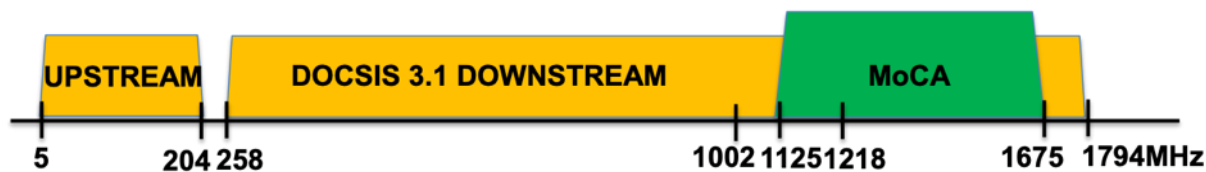
Figure 26 – DOCSIS 3.1 and MoCA signals could share the same frequency spectrum
