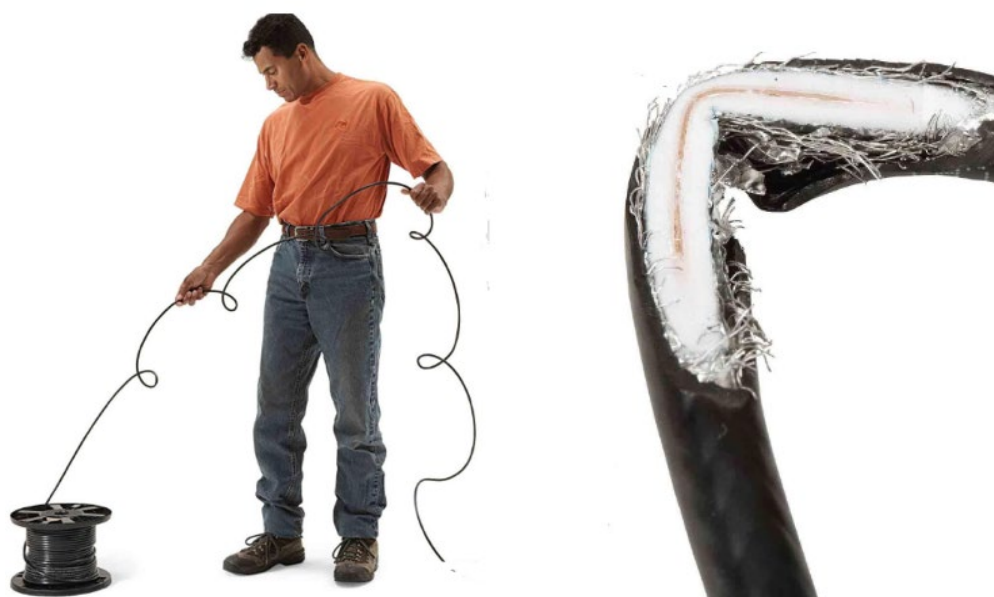
Figure 80 – Cross-section of kinked coaxial cable
