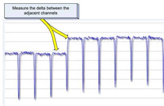
Figure 18 - Adjacent misalignment in SC-QAM channels at a CPE
