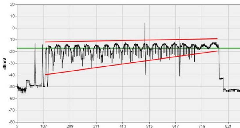
Figure 55 – Non-uniform standing wave with high frequency attenuation
