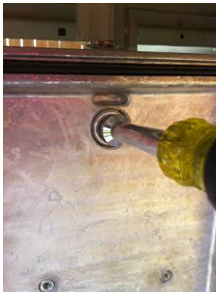
Figure 39 – CPD noise (top) caused by loose seizure screw (bottom) on amplifier output
