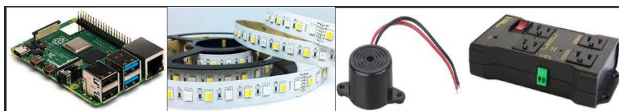
Figure 4 - Raspberry Pi, LED Strip, Buzzer, IoT Relay
