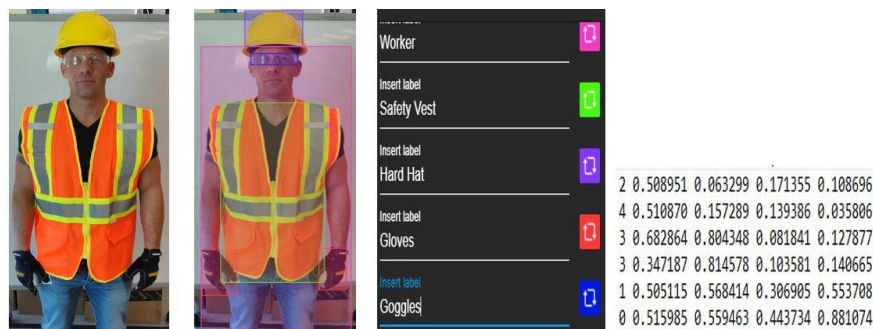
Figure 13 - Worker, Annotated Worker, Classes, and YOLO Coordinates
