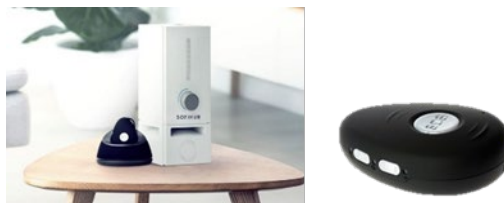
Figure 22 - SOFIHUB home and beacon assisted living device and safety pendant
