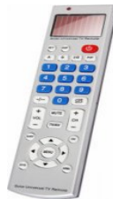
Figure 6 - Remote Control with Solar Cell
