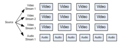
Figure 2 - ABR with audio durations different than video
