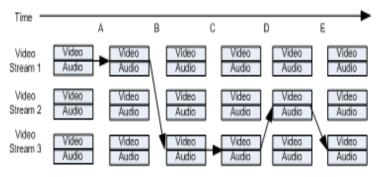
Figure 4 - ABR chunk switching
