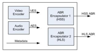
Figure 8 - Unified Transcoder/Encapsulator
