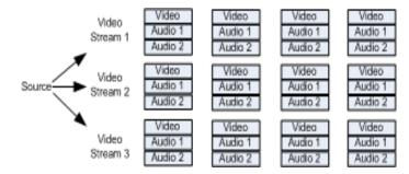
Figure 3 - ABR with interleaved audio and video streams
