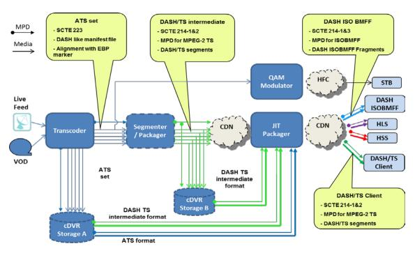
Figure 10 – DASH Service Reference Architecture Diagram
