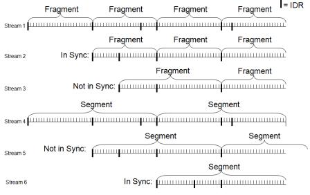
Figure 7 - Fragment and Segment Sync/Alignment
