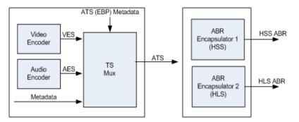
Figure 9 - Separate Transcoder/Encapsulator with ATS in between
