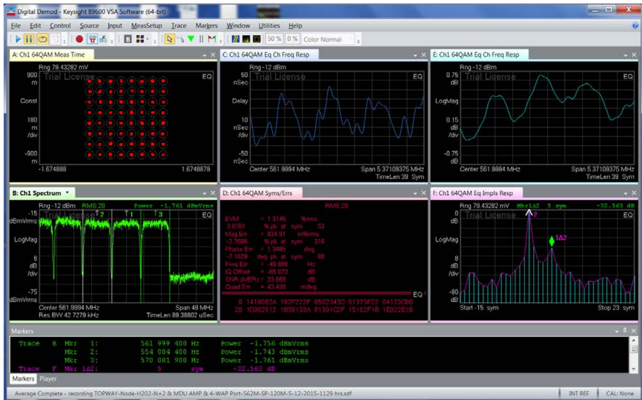
Figure 4a – Forward path direction micro-reflection example – carrier frequency = 562 MHz
