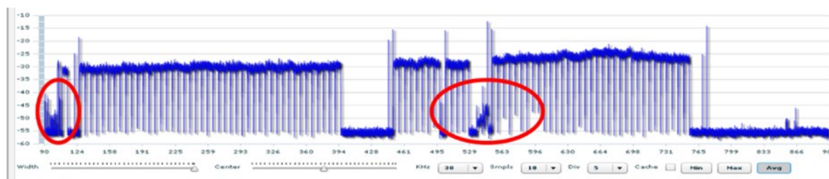
Figure 37 - Full band capture display showing relatively flat frequency response. Ingress is also visible (circled in red). Graphic courtesy of Comcast.
