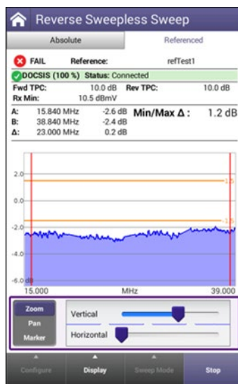
Figure 47 - Another example of commercial implementation of upstream active spectrum frequency response derived from pre-equalization coefficients. Graphic courtesy of Viavi Solutions.
