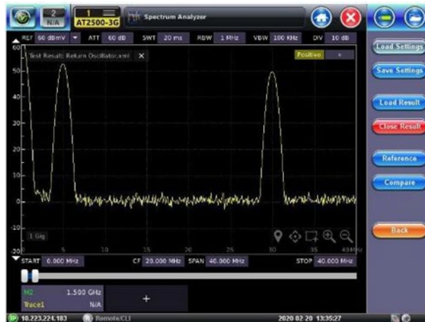
Figure 31 - Return path alignment carriers at 5 MHz and 30 MHz from a Viewsonics VSOSC-2F Dual Frequency Oscillator (photo courtesy of Jonathan Jurta, Atlantic Broadband).
