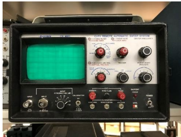
Figure 16 - Avantek sweep receiver, which included spectrum analyzer functionality (photo taken at The Cable Center; used with permission of the Barco Library, The Cable Center ).
