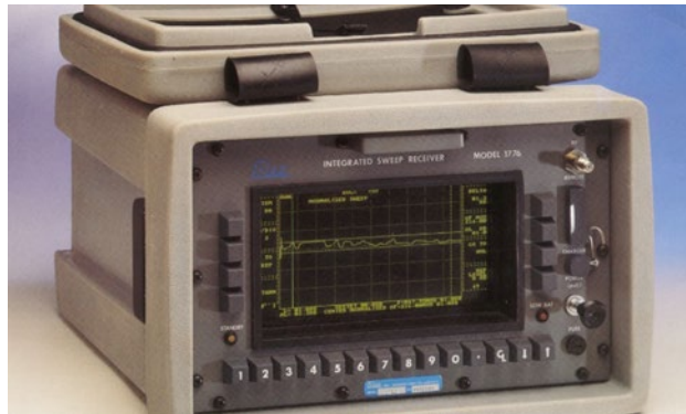
Figure 19 - CaLan model 1776 sweep receiver (photo from an old CaLan product brochure, courtesy of VeEX).
