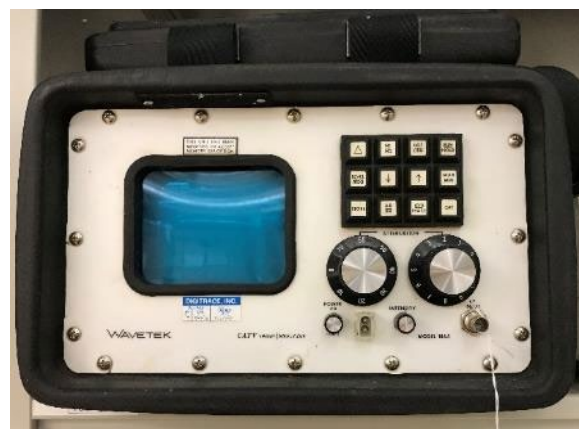
Figure 14 - Wavetek 1865 sweep receiver (photo taken at The Cable Center; used with permission of the Barco Library, The Cable Center ).
