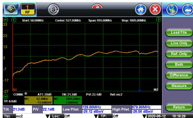
Figure 59. Another example of low-end rolloff (courtesy of VeEX).
