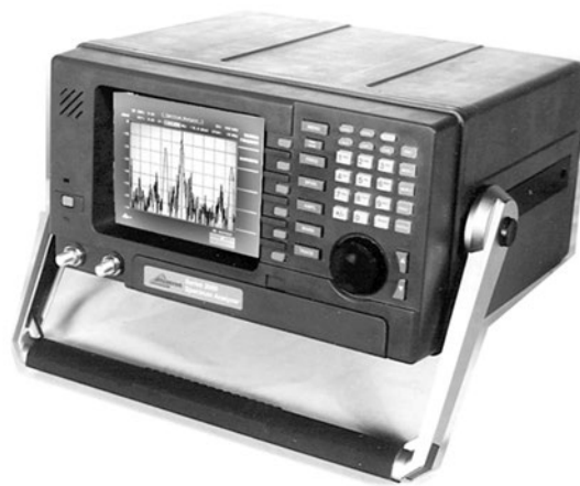
Figure 18 - Avantron AT2000R spectrum analyzer with integrated low-level sweep receiver (courtesy of Bernie Cadieux).
