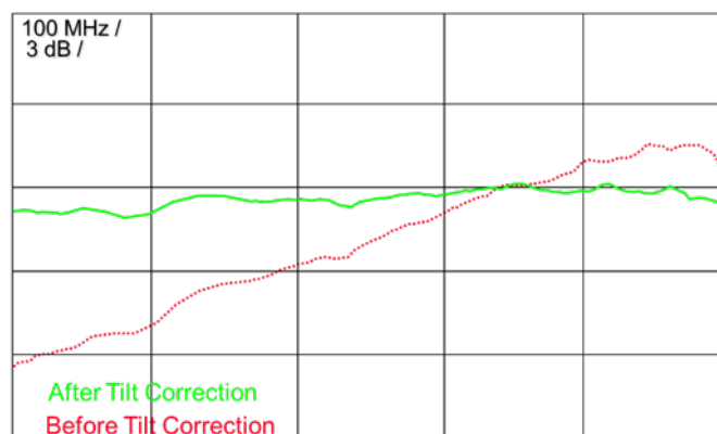
Figure 6 - Sweep receiver tilt compensation example (graphic from a Wavetek Wandel Goltermann training presentation; courtesy of Viavi Solutions).
