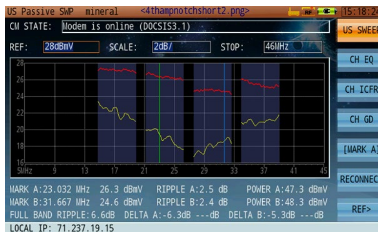
Figure 46 - Example of commercial implementation of upstream active spectrum frequency response derived from pre-equalization coefficients. This screen shot shows a captured reference (red traces) and a response trace from another test point affected by an impairment (yellow traces). Graphic courtesy of Deviser Instruments.
