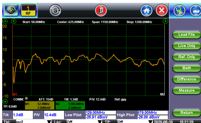
Figure 52. Another standing wave example (courtesy of VeEX).
