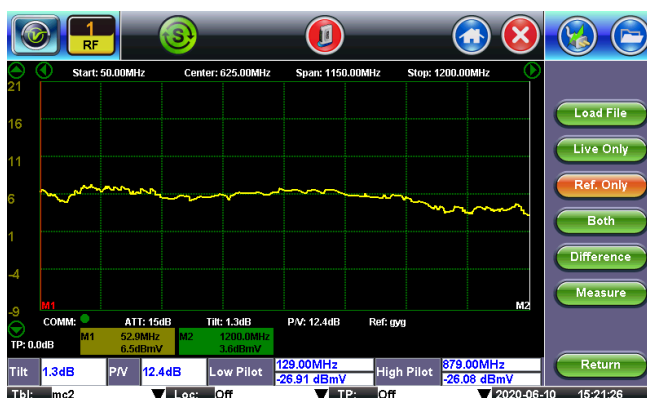
Figure 53. Same swept spectrum as Figure 52, but without the impedance mismatch that caused the standing wave (courtesy of VeEX).
