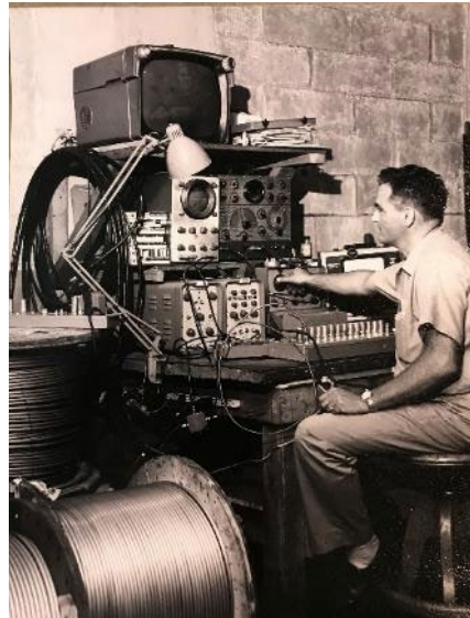
Figure 11 - Early bench sweep (photo used with permission of the Barco Library, The Cable Center).
