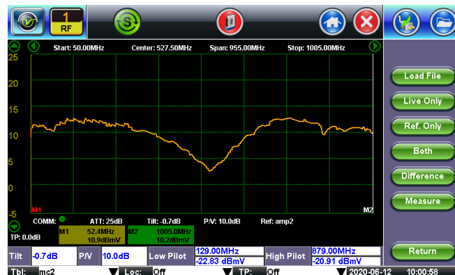
Figure 50. Another example of a frequency response suckout (courtesy VeEX).
