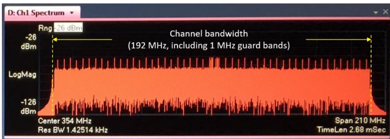
Figure 16-43: Spectrum Analyzer Screen Shot Of A 192 Mhz-Wide Downstream OFDM Signal.
