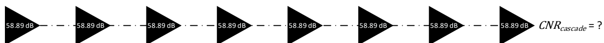
Figure 15 - What is the CNR at the end of this cascade of identical amplifiers?
