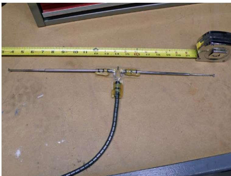
Figure 24. Homemade half-wave dipole antenna using telescoping elements. This particular antenna was designed to be used over a frequency range from about 100 MHz (elements fully extended) to 300 MHz (elements fully collapsed).
