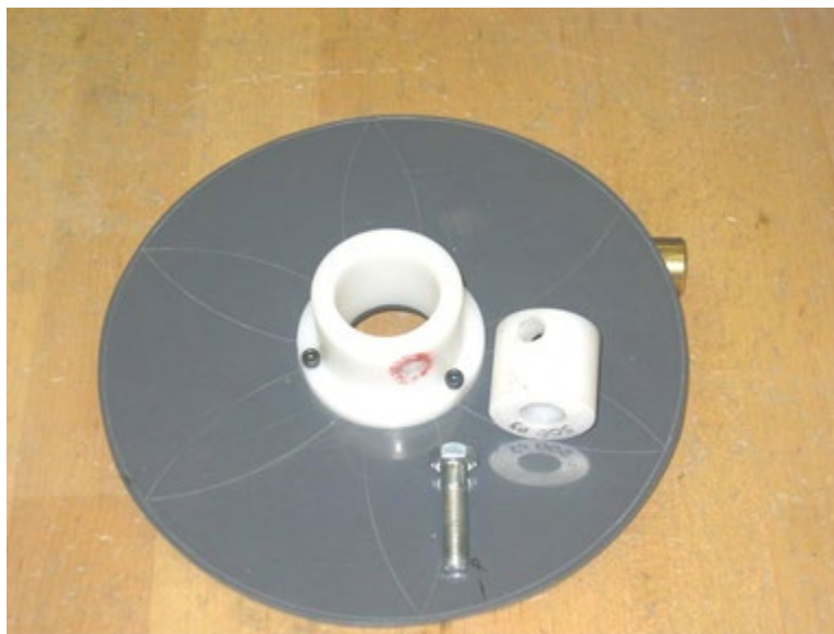
Figure 6 - Rear View Of Degree Wheel And Related Parts
