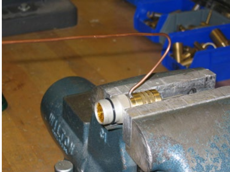
Figure 5 - Connector Body With Pointer And Retaining Nut In Vice
