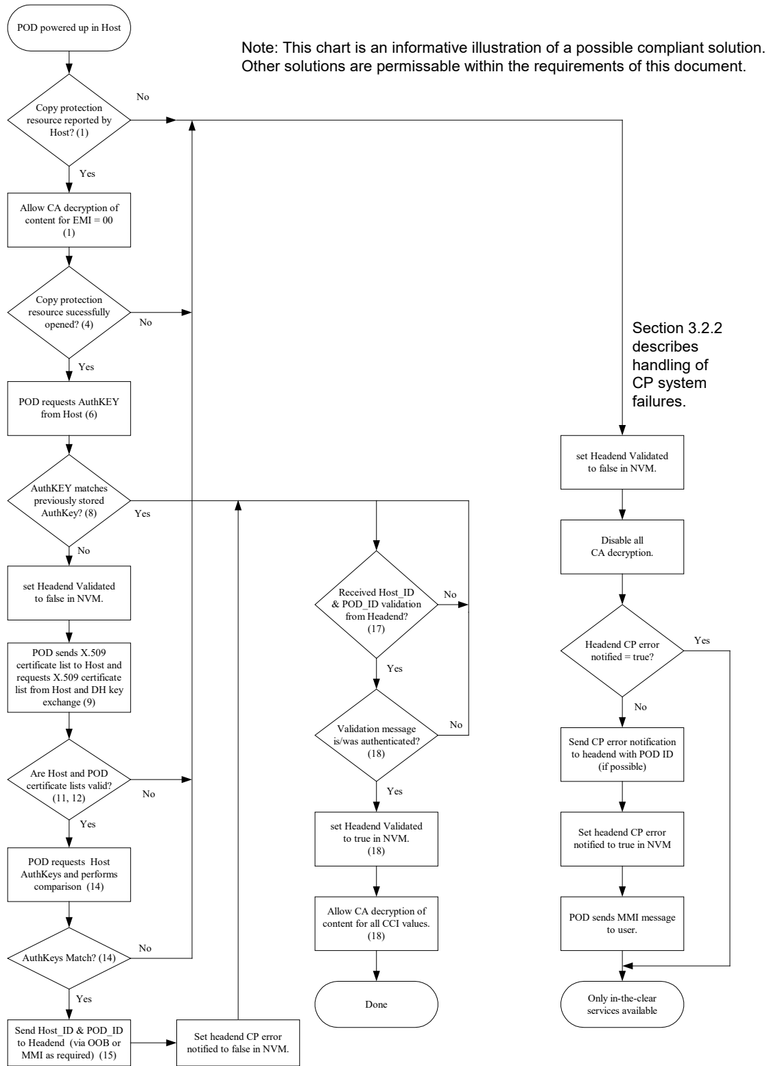
Figure 3.1-A POD-Host CP Operation
